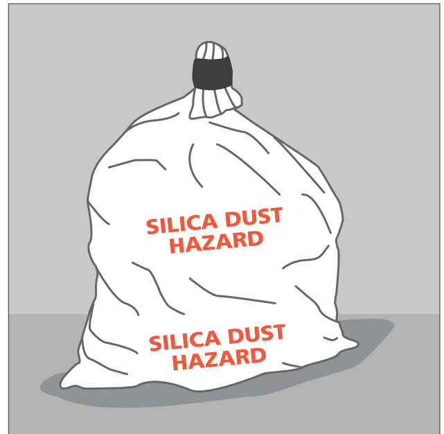
Figure 16: Waste contaminated by silica dust needs to be bagged and labelled
