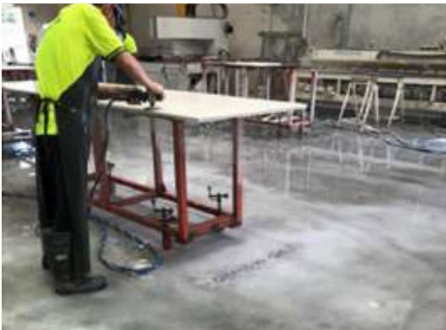
Photo 1 — Wet polishing of engineered stone
