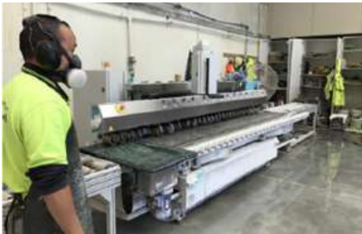
Photo 2 — PPE/RPE examples in stone fabrication
